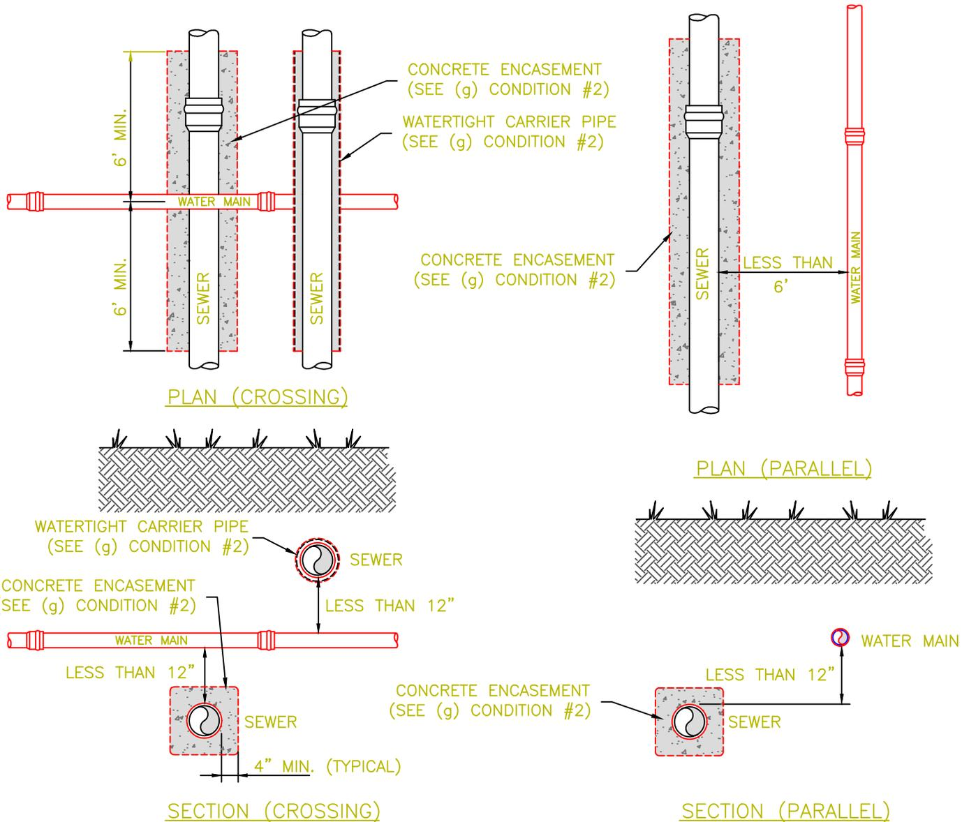
SEWERS AND FORCE MAINS SHALL BE LAID AT LEAST TEN FEET (OUTSIDE TO OUTSIDE) HORIZONTALLY FROM WATER MAINS.
