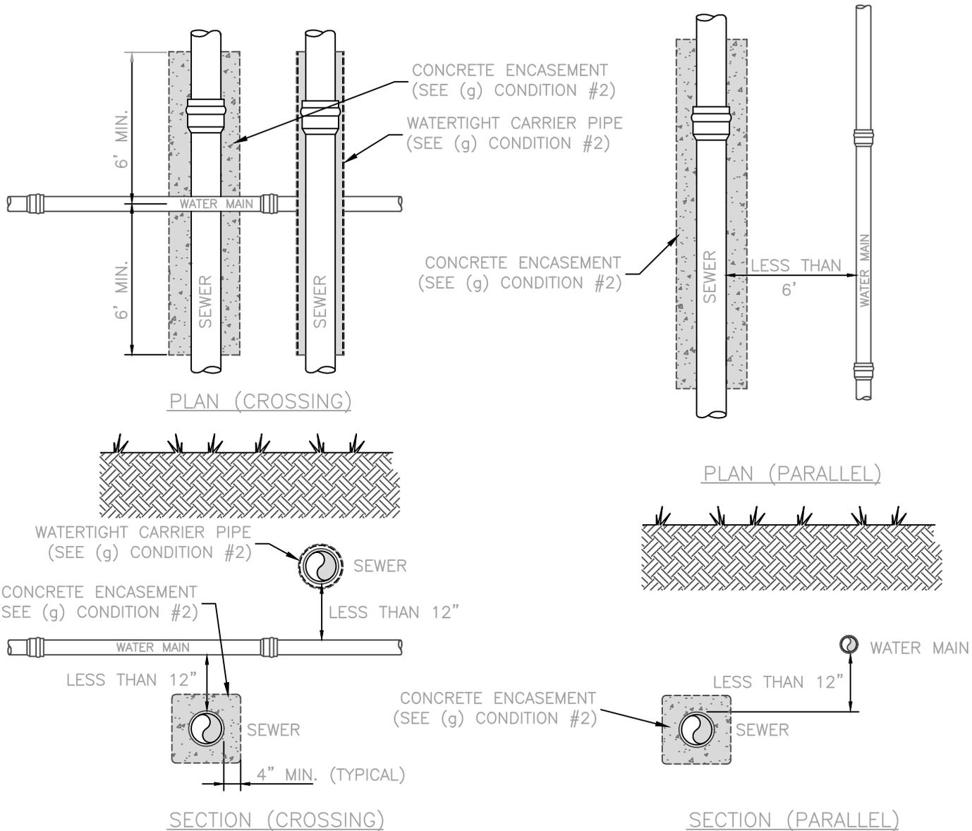
SEWERS AND FORCE MAINS SHALL BE LAID AT LEAST TEN FEET (OUTSIDE TO OUTSIDE) HORIZONTALLY FROM WATER MAINS. PROVIDED THE APPLICANT DEMONSTRATES THERE IS NO REASONABLE ALTERNATIVE, THE CITY MAY APPROVE SMALLER HORIZONTAL SEPARATION DISTANCES FOR SEWERS IF ONE OF THE FOLLOWING CONDITIONS IS MET:
